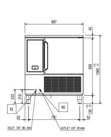
Drain Electrical inlet (power) ΕI Refrigerant Outlet
